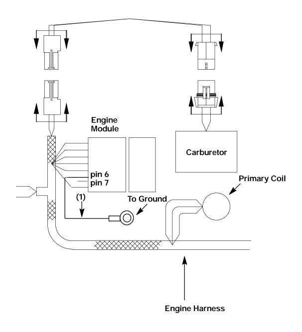
FIG. 1 - Pictorial for LP Engine Module Ground
